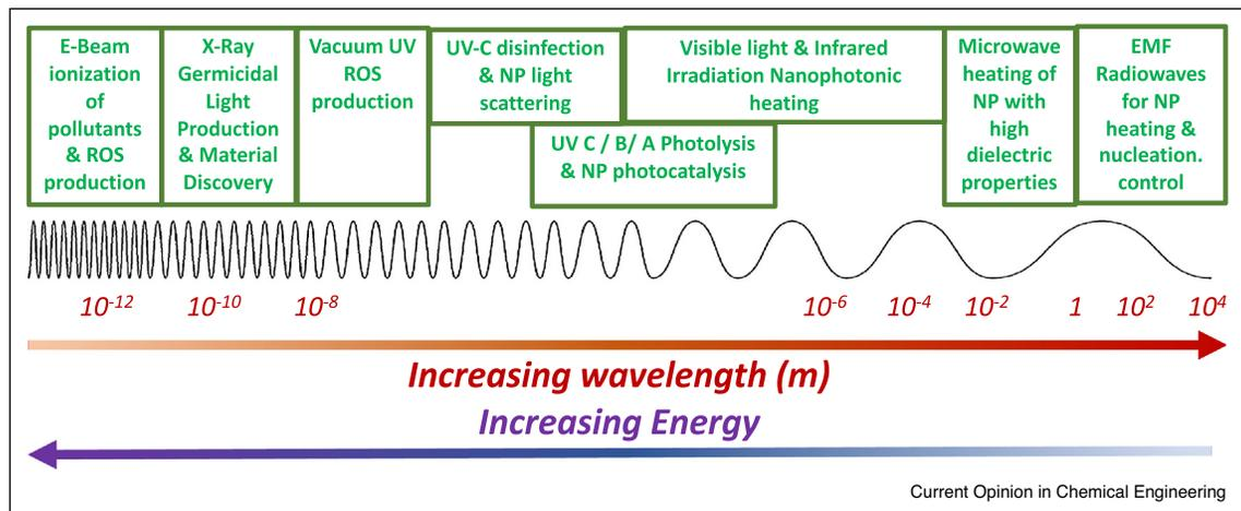
Electromagnetic spectrum ranges that can be used in conjunction with nanotechnology to enable disinfection, pollutant oxidation or reduction, and localized thermal driven desalination (frequency ( $f$ , Hz) =  $C/\lambda$ , where the  $C$  is speed of light ( $3 \times 10^8$  m/s) and  $\lambda$  is wavelength of energy (m); Hertz (Hz) have units of  $\text{sec}^{-1}$ ).
